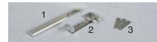
1. Sampling holder 2. 5-sample holder 3. Sample cells
