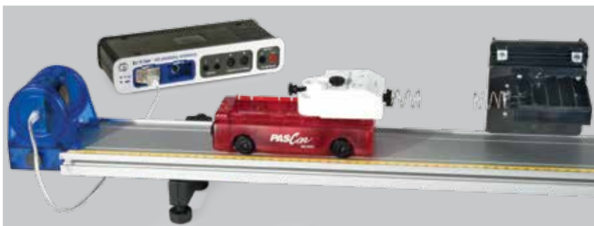
Wireless Force Acceleration Sensor (PS-3202) in cart collisions with fixed spring bumper on Force Bracket
