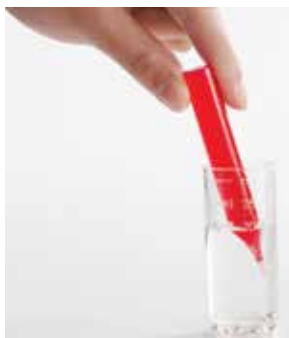
The sample instantly flows into tube, mixing with the reagent.
