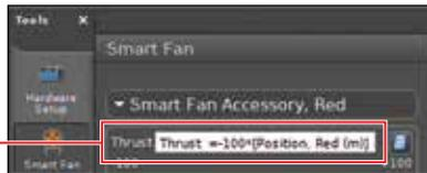
This will cause the fan to blow harder as the cart moves down the track, causing the cart to reverse, and eventually the fan will reverse when the Position becomes negative, accelerating the cart in the positive direction.
